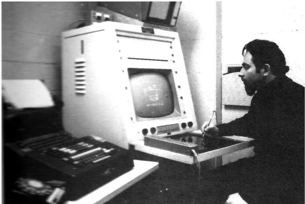
Fig 11.1: A typical interactive computer-mediated animation console. The author is drawing with the stylus on the tablet and observing the result on the display scope. On this display, movies are played back in real time. The typewriter is also used for communication between animator and computer. The knobs under the display help to make fine adjustments to images. The toggle switches on the tablet are used to set line texture densities, playback speeds and other parameters.
